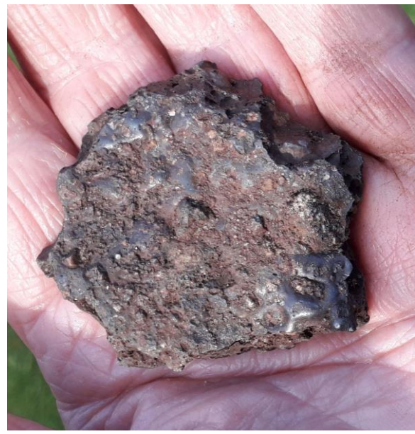
Fig 5. A small piece of slag from Beeston Regis. The smooth, formerly molten parts catch the light.
